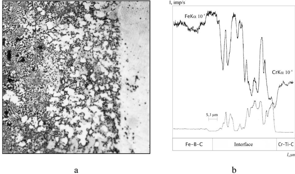
**Fig. 4. Microstructure,  $\times 400$  (a) and distribution of components at (Fe–3.1B–0.1C)/(Cr–20Ti–10C) interface (b).**
