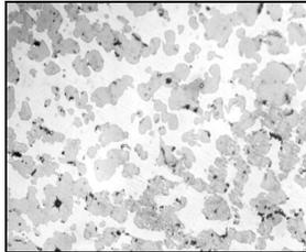
Fig. 1. Microstructure of Cr–20Ti–10C alloy,  $\times 200$
