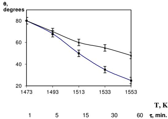
Fig. 3. Wetting angles of Cr–20Ti–10C alloy by Fe–3.1B–0.1C melt: 1 – as a function of temperature T; 2 – as a function of holding time  $\tau$ .
