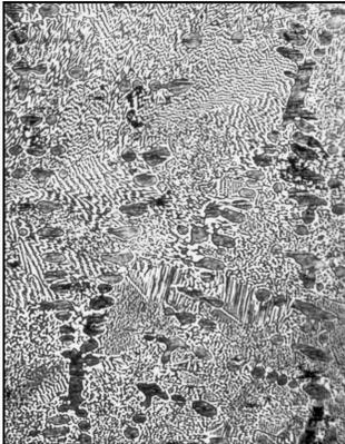
Fig. 2. Microstructure of wetting Fe–3.1B–0.1C alloy,  $\times 400$ .
