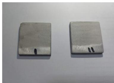
Fig. 8. The AlSi templates with the protective coatings.
