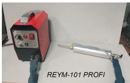
Fig. 7. General view of the device for the cold gas-dynamic spraying.
