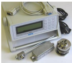
Fig. 3. Quartz film thickness gauge (five version) QFTG-5.
