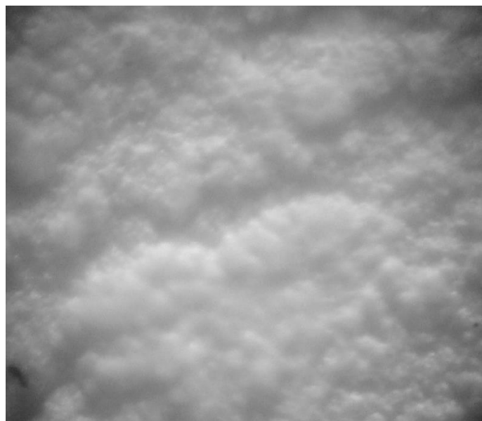
Fig. 3. Optical micrograph of the ZnO layer obtained by chemical precipitation ( \times 100 ).
