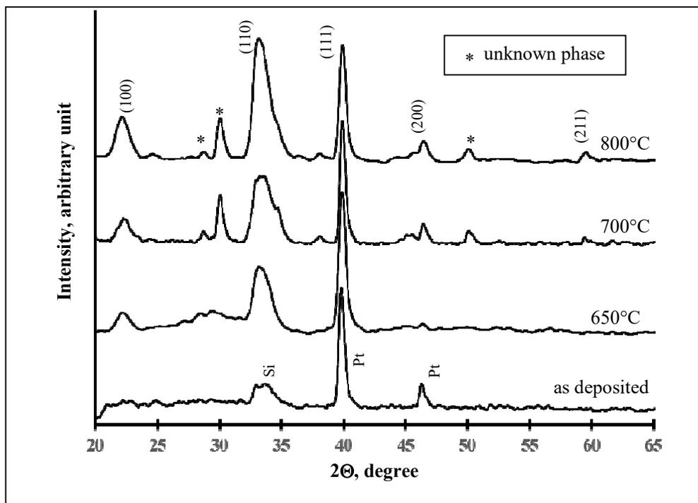
Fig. 1. XRD patterns of as deposited NBT thin films and NBT thin films annealed in air at  $T = 650^{\circ}\text{C}$ ,  $700^{\circ}\text{C}$  and  $800^{\circ}\text{C}$ .
