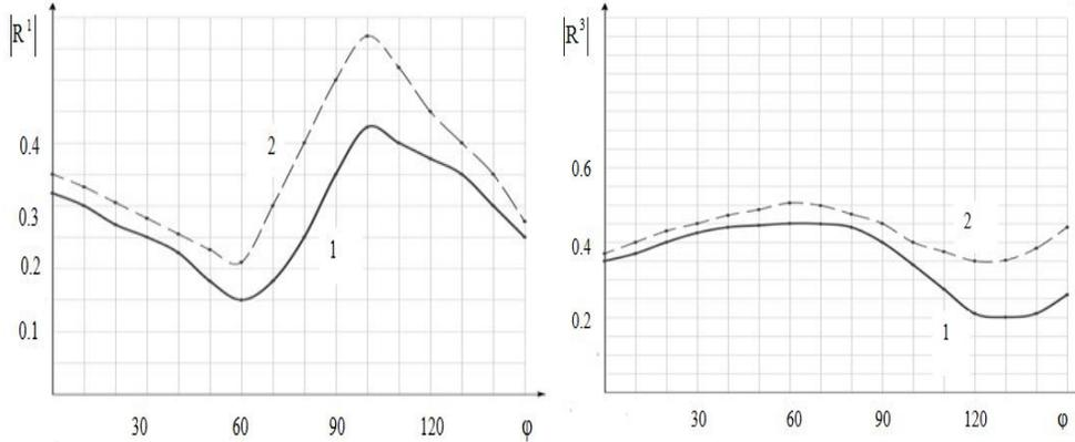
Fig. 3. Dependence of  $|R^n|$  on the phase shift  $\varphi$  for a fixed  $rz1/\lambda$  and different  $rz2/\lambda$ :  $N=5$ ;  $b=0.6\lambda$ ;  $a=0.1\lambda$ ;  $rz1=0.25\lambda$ ;  $c=0.15\lambda$ ; 1 –  $rz2=0.45\lambda$ ; 2 –  $rz2=0.5\lambda$ .
