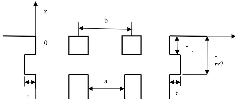
Fig. 1. The finite linear antenna array in the plane ZOY.
