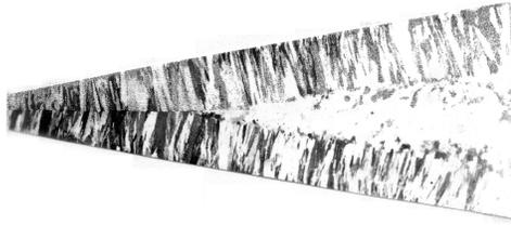
Fig. 5. Microstructure (x300) of steel P-18 obtained in wedge casting form.
