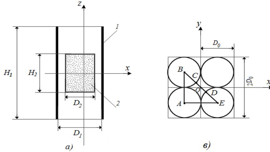
**Fig. 1. Solenoidal coil (1) contained the sampler (2) filled with powder:**  $H_1$  and  $D_1$  are height and interior diameter of the solenoidal coil,  $H_2$  and  $D_2$  are height and interior diameter of the cylindrical sampler (a); powder particles arrangement in section  $xy$ , perpendicular to the solenoid axis for dense matrix particles packing (b).
