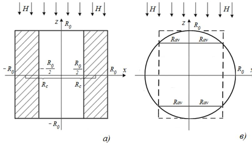
Fig. 3. Axial sections of the cylindrical particle (a) and spherical particle (b).
