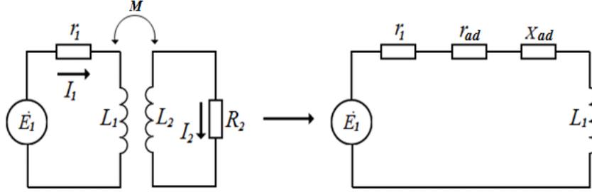
Fig. 4. Equivalent scheme representing the interaction of the solenoidal coil field and the field of eddy current induced in the particle of powder.
